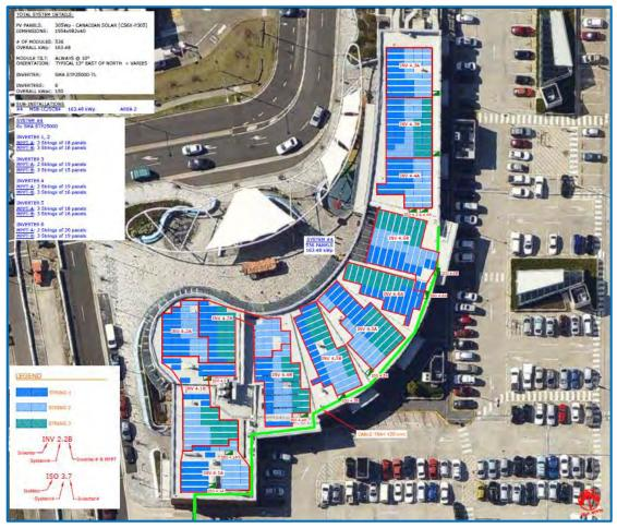
SMA inverters allowed flexible electrical design around the challenging physical panel layout design. Electrical string configurations to match panel layouts on challenging roofs areas.
