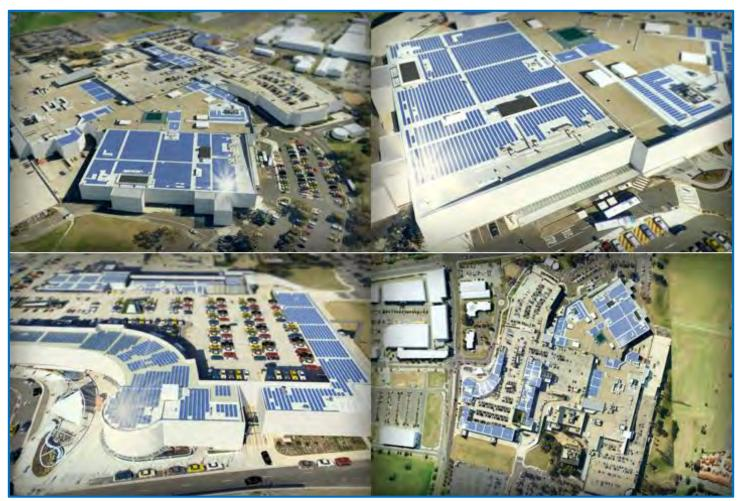
The Todae Solar Engineering department initially created an accurate 3D design of the building and surroundings adding the 3992 panels and the mounting.
