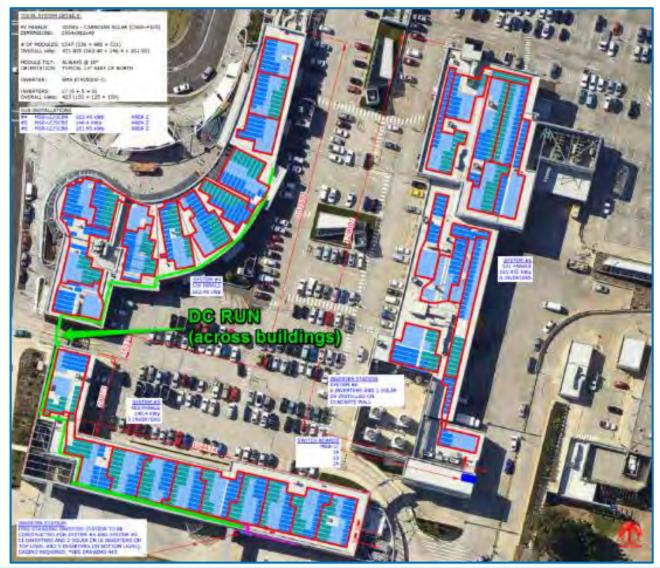
Todae Solar managed to create a string and cable configuration to minimise the DC losses to 1.5%, well under the 3% maximum required in AS5033:2014.
